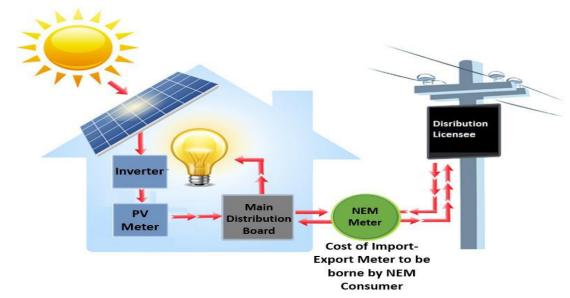
The diagram of the connection between the consumer's solar PV system and the DL distribution system
