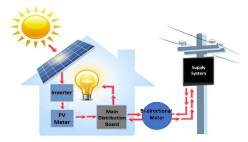
Figure 3: The connection of a solar PV installation to the consumer electrical installation
