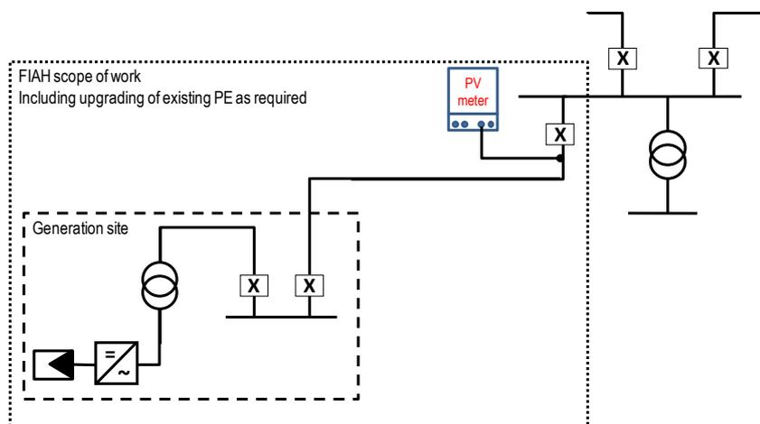
Fig 8.5 - PV connections diagram at PE
