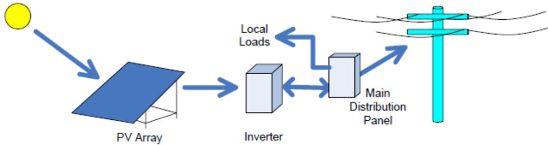
A1 – Grid connected PV systems with no storage
