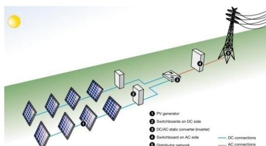
Large scale PV connected to distribution network [2]
