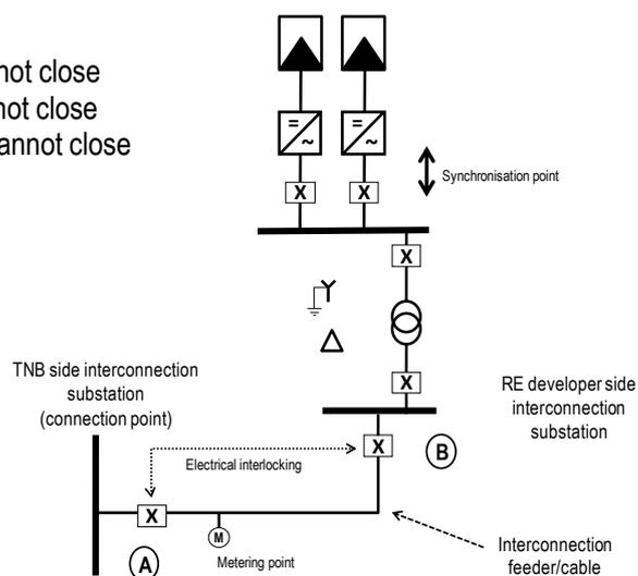
Fig 6.1 Interlocking & synchronization of MV system
