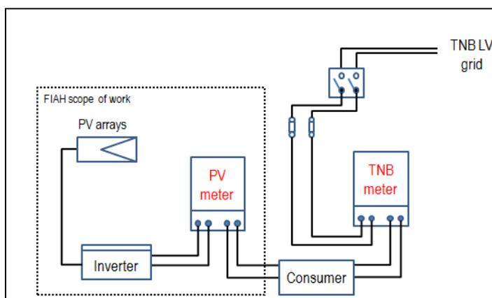
Fig 8.4 – PV indirect connections diagram for LV
