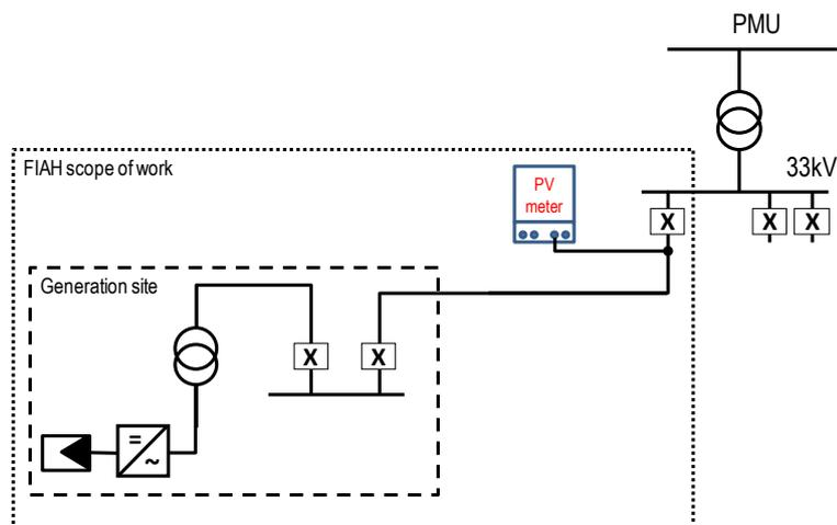
Fig 8.7 – PV connections diagram at PMU (33kV)
