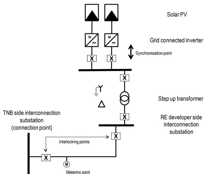
Fig 4.1 Proposed interconnection on MV system
