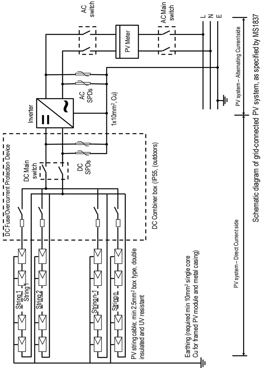
Schematic diagram of a grid-connected PV system (single-phase) as specified in MS IEC 1837
