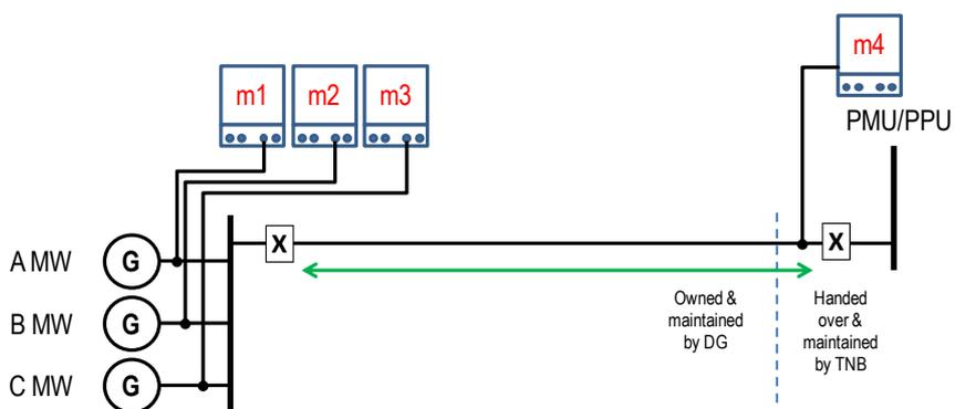
Fig 8.8 – Multi-feed configuration
