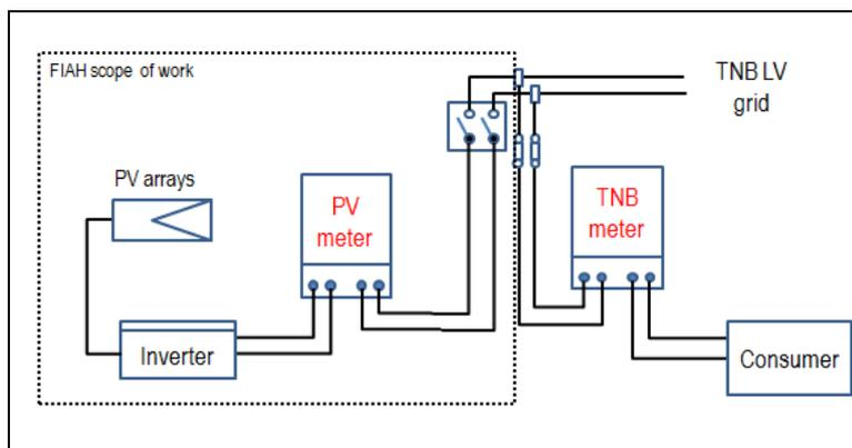
Fig 8.3 – PV direct connections diagram for LV
