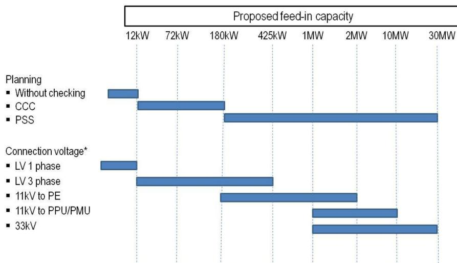
**8.5 Type 1 – LV single phase** : Type 1 is applicable for PV < 12kWp. Typically for residential, terrace units. Connection is by single phase.
