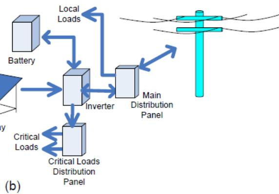
A2 – Grid connected PV systems with storage using (a) separate PV charge control and inverter charge control, and (b) integrated charge control
