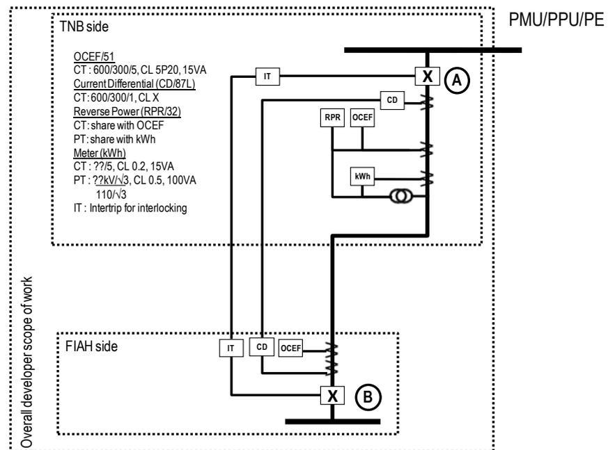
Fig 8.9 – Interconnections diagram between TNB and FIAH
