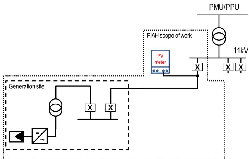
Fig 8.6 –PV connections diagram at PMU/PPU (11kV)
