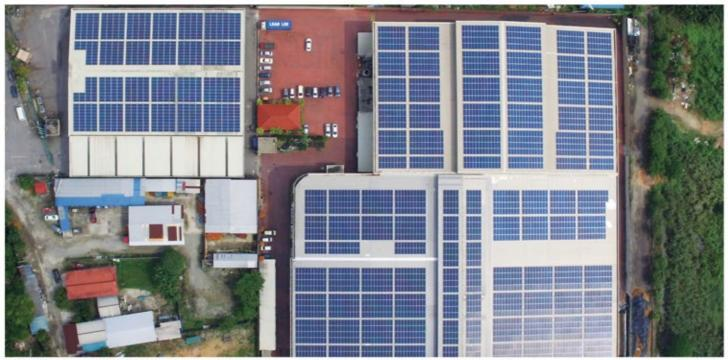
NEM 1.0 programme - a 675.3kW solar PV system installed on the buildings of Lean Lee Trading Company Sdn. Bhd.
