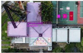
**Solar Installation** of **15.4 kWp** under the Net Energy Metering Scheme with total of **28 nos PV module** monocrystalline at the roof top with savings up to **RM800+ per month** – status in progress
